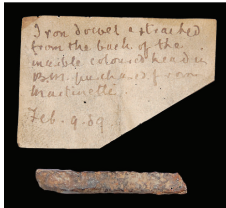
Fig. 2. The iron dowel (GR 1884,0617.2).
